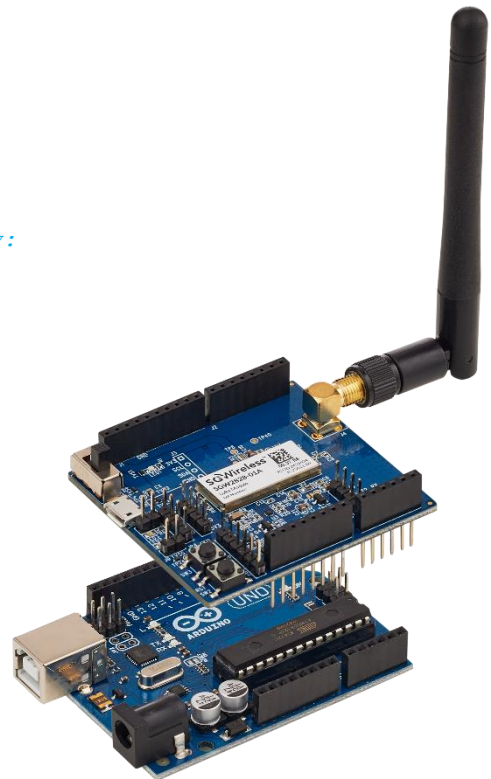
Figure 18: SGW2828-EVK and Arduino UNO Connection
