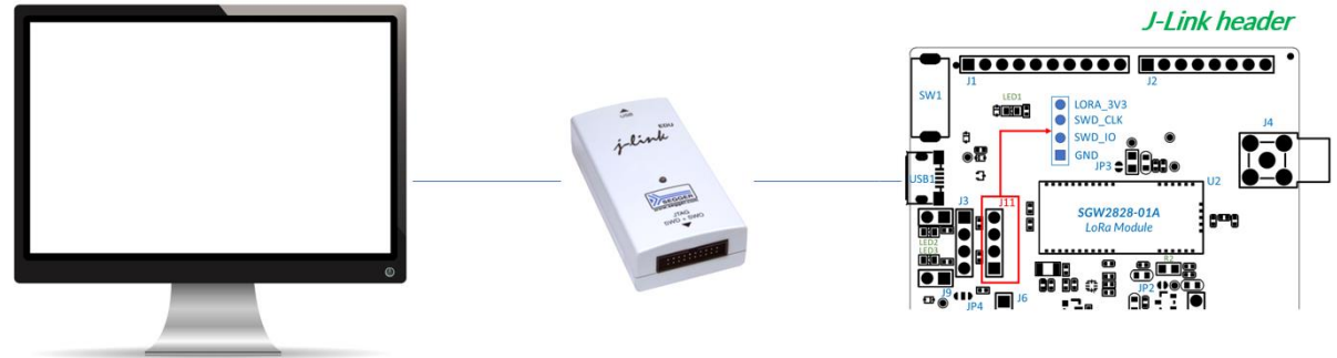
Figure 14: SGW2828-EVK to PC Connection via J-Link Kit
