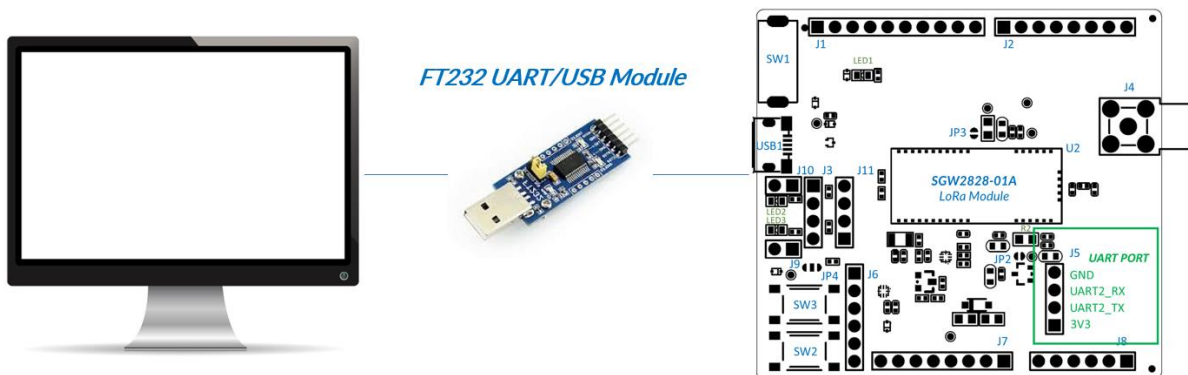
Figure 17: SGW2828-EVK to PC Connection via EVK UART
